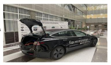
The centre has already got working prototypes of hydrogen power systems of their own design, which allow doubling the mileage of an electric car (about 1000 km). The collaboration plans include technological improvement of the existing developments of the company jointly with the university and subsequent mass production. Currently, they are working on modifications of light duty and passenger electric vehicles with hydrogen power systems.
