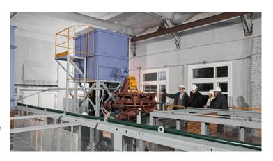
The Educational and Production Laboratory of Hydraulics and Hydromechanics has unique stands and an operating hydraulic unit. Experts note that there are no analogues of this laboratory not only in Russian educational institutions but also abroad. For example, the hydroelectric unit installed in the lab is an accurate, 10 times smaller, copy of the hydroelectric unit of the Sayano-Shushenskaya HPP.
