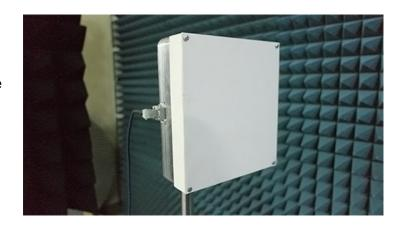
The antenna array will be an integral part of the new mobile satellite communications stations of JSC "NPO Radiosvyaz" intended for satellite broadcasting in Ka and Q bands.
