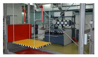
The authors of the idea had a task of creating the universal, but small-sized unit, which imitates side shocks and falls. Such equipment, due to the efficient use of the testing laboratory area, can reduce the cost of the tests themselves. At the same time, the unit can be used for testing both cardboard, plywood, wooden boxes and bottle products, containers for liquid and bulk materials, construction bags. It took six months to implement the idea.
