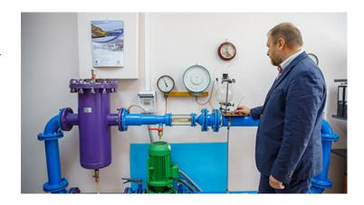
The authors of the research developed a technology for fresh water production by cavitation, a phenomenon in which rapid changes of pressure in a liquid lead to the formation of small vapor-filled voids (cavitation microbubbles). The microbubbles collapse causes temperature rise to 15 thousand degrees Celsius, generate intense shock waves up to 10 atmospheres and needle-like jets, in which water moves at a speed of up to 500 meters per second.
