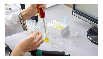
The main component of the biosensor, SibFU scientists work with, is a biomodule, which is an enzyme of luminous organisms. Under favorable conditions enzymes emit light, which are indicated by a special device — luminometer. However, this glow is reduced in the presence of toxic substances. According to the intensity of light emitted, scientists can assess the quality or safety of a product.
