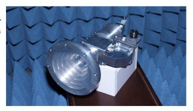
The feeder is a part of a satellite communication station. It is installed in a regular place of attachment on the satellite antenna and is used to transmit and receive radio waves in multiple frequency bands. Receiving and transmitting modules are connected to the feeder that allows boosting the signal and registering it by measuring devices.
